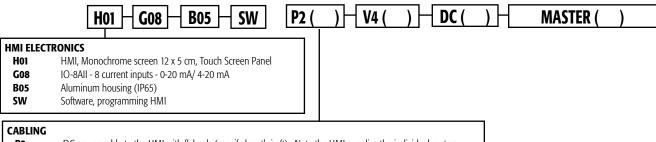
P2 DC power cable to the HMI with flyleads (specify length in ft). Note the HMI supplies the individual meters
